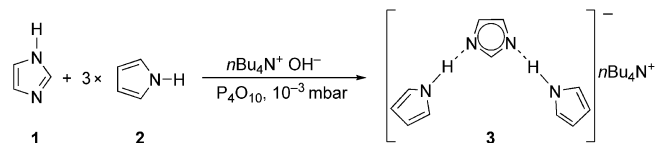
Scheme 1. Preparation of tetrabutylammonium imidazolate-dipyrrole 3 .
